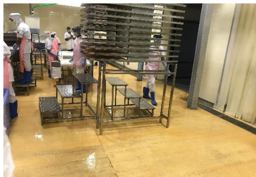
Fig 6-Placement of Equipment for easy and effective cleaning
