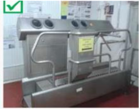
Fig26: Automatic hand-washing and foot cleaning system
