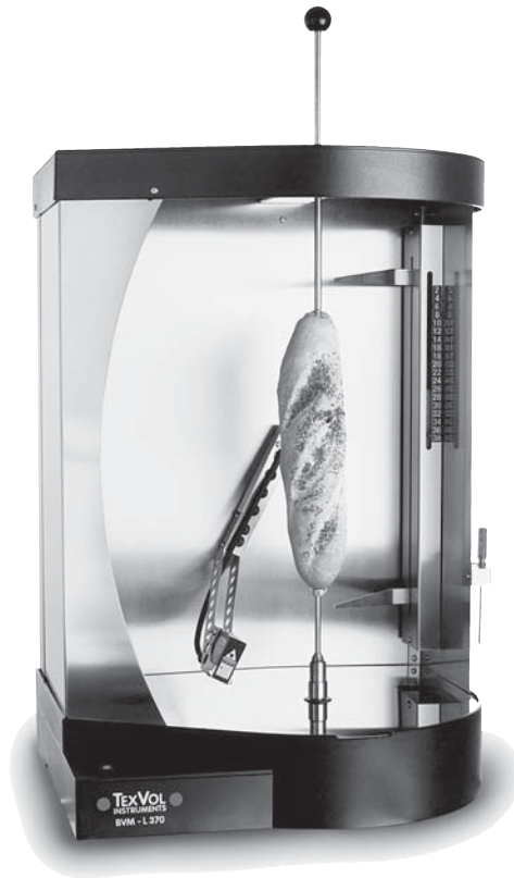
Figure 2.4 TexVol instrument for volume measurement. Reproduced with permission of TexVol Instruments AB, Viken, Sweden.
