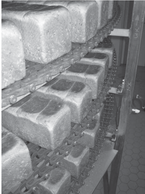
Figure 7.7 Bread in a commercial spiral cooler. Reproduced with permission of Frank Roberts & Sons Ltd.
