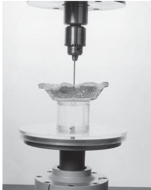
Figure 2.6 Puncture testing of composite apple pies.
