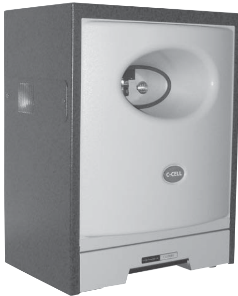
Figure 5.4 C-Cell instrument for assessing crumb cell structure. Reproduced with permission of Calibre Control International.
