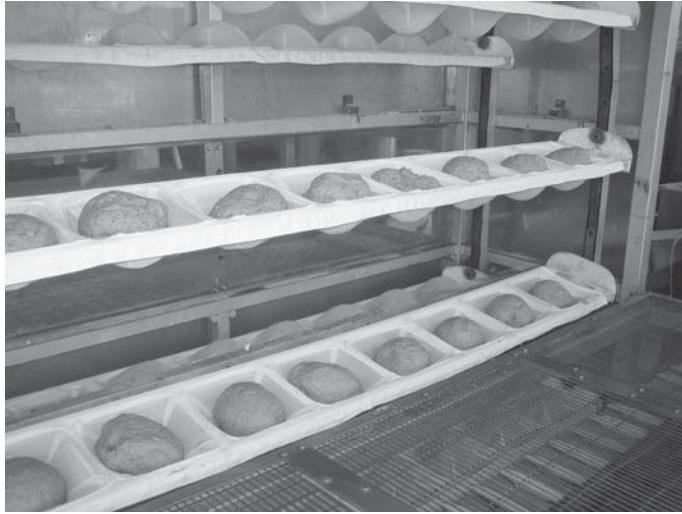
Figure 6.7 Resting of dough pieces in a commercial first prover. Reproduced with permission of Frank Roberts and Sons Ltd.
