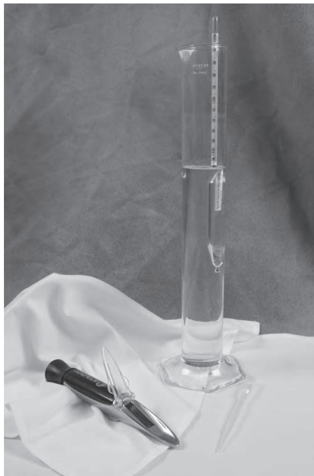
PHOTO 8.3 A refractometer (on the left) and hydrometer (on the right) in use Photo by Aaron Seyfarth
